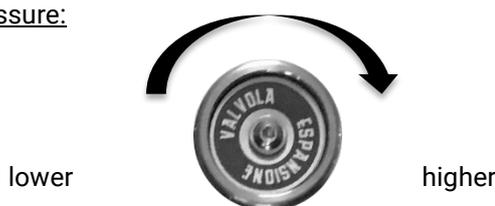
You can reduce the brewing pressure by turning the screw anti-clockwise and increase it by turning it clockwise.
